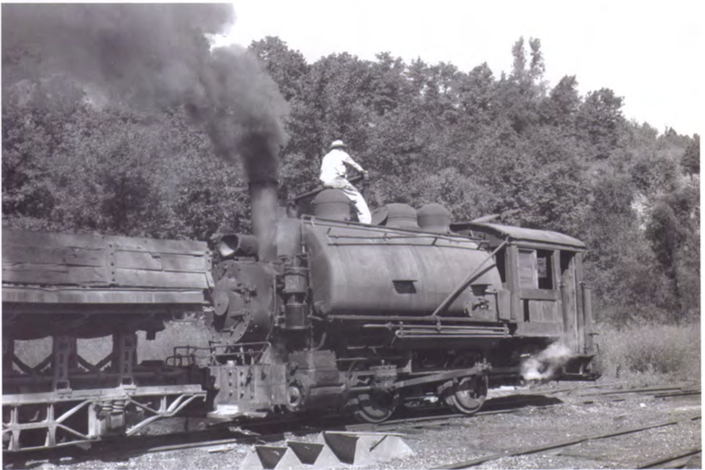
Top: Dresser Trap Rock nos. 3 and 5 are tied up for the day near the enginehouse. These 0-4-0 saddle tank locomotives had seen better days when photographed on July 18, 1960. Bottom: Dresser Trap Rock no. 4 gets a drink of water before its last trip of the day. The sand domes had long been disconnected, but made a handy seat for the engineer while he filled the tank. Both photos - Larry Easton.
